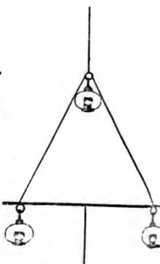
Four lanterns and two yards, each not less than four feet long, will be sufficient — as only one signal will be used at night. These signals may be made with any lanterns, showing either white, or any colour, but *alike*. *Red is most eligible*. Lamps are preferable to candles. The halyards should be good rope, and protected from chafing. The lanterns should hang at least three feet apart.
